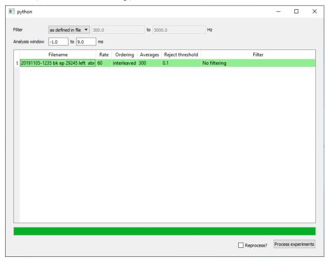
To load files, drag-and-drop the folder containing the ABR data onto the GUI. Unprocessed files are shown with a white background. If the file has already been processed, it will be shown with a green background. Once you have loaded the files you wish to process, you can specify the filter and epoch settings. By default, the filter settings specified during acquisition will be loaded from the file. If you wish to reprocess a file, you need to check the "reprocess files".
